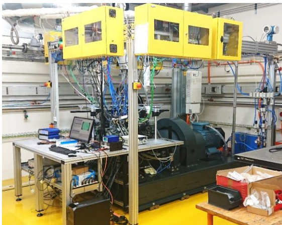
Fig. 5. The Flex-OeCoS – a novel optically accessible test rig for the investigation of advanced combustion processes under engine-like conditions
