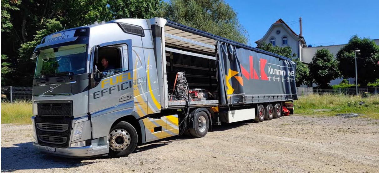
Fig. 4. Truck Fueled with Liquefied Biogas and with FTIR-PEMS Measurement Installation (Source: AFHB)
