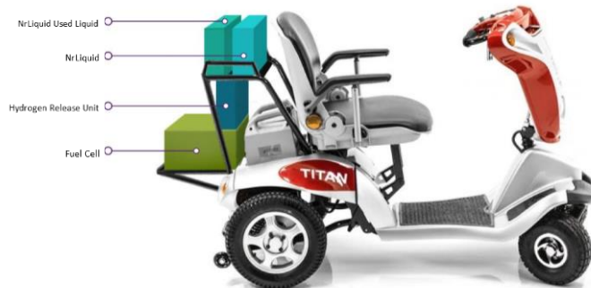
Fig. 2 A small vehicle continuously charged by NrgStorEdge
