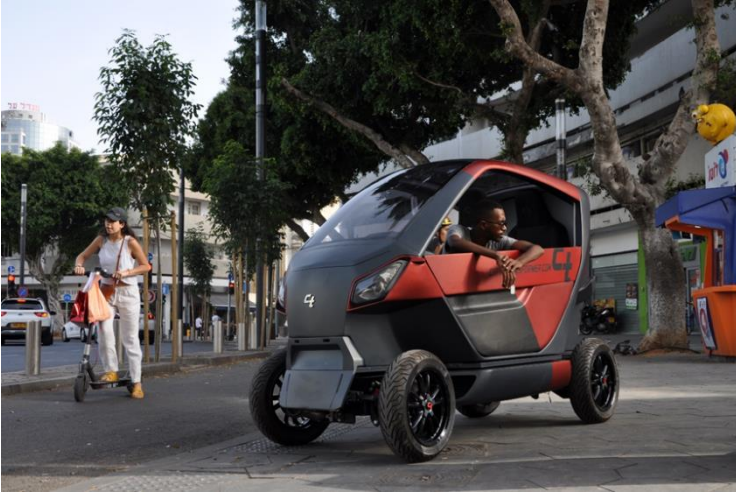
Fig. 3 The City Transformer folding vehicle is only 1 meter wide and can go 90 Km/h
