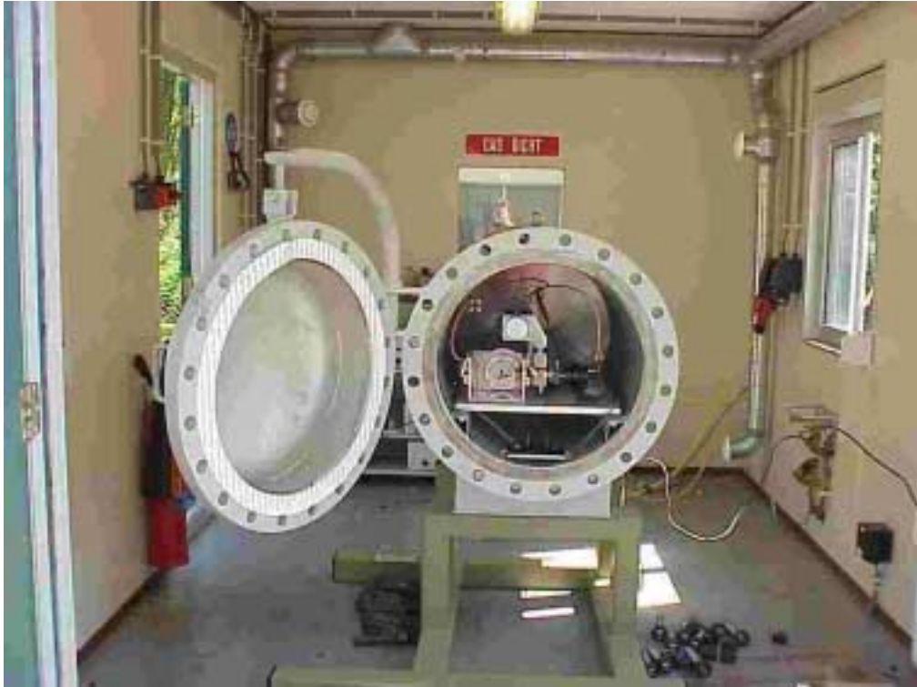
Figure B.2: Inside of Tribometer (Tank cover removed)
