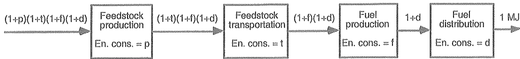
Fig. B.3 Energy consumption calculation method for the first four steps of the total well to wheel fuel chain.
