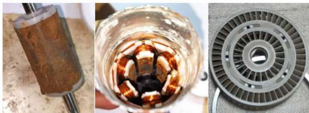
Corrosion and wear parts of methanol pump
