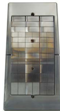
Tungsten tiles of different shapes for the study of tritium (Source: NFRI, Korea)
